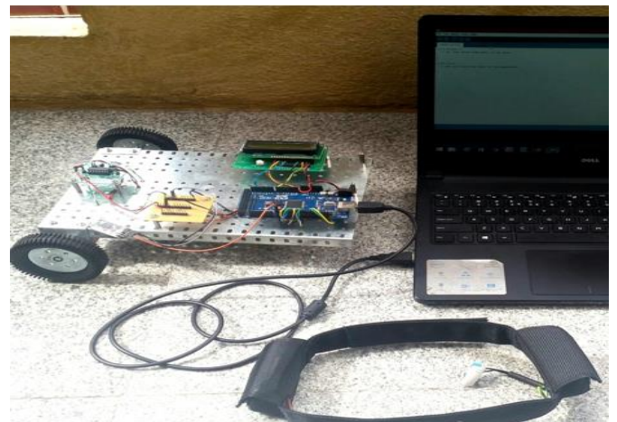
Figure xii: The Brain sensor band and the Pluguino powered car
