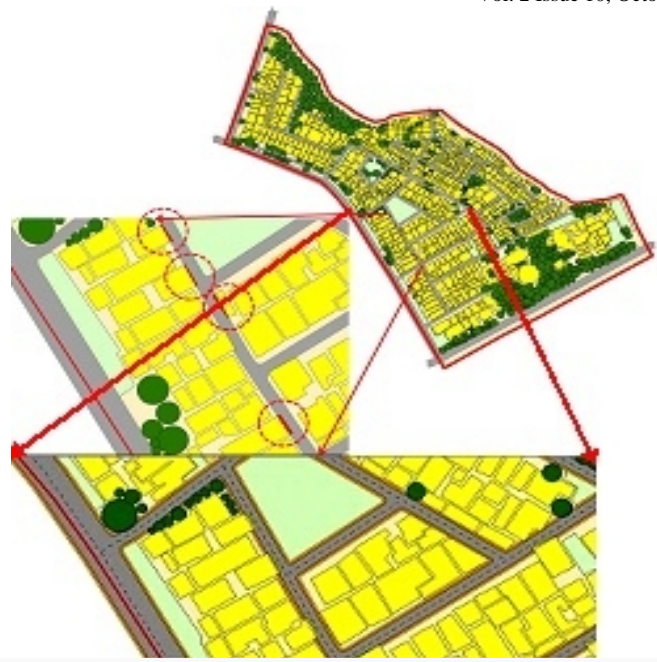
Figure 8: Identified encroached built cover on road and 1.2m buffer along road for footpath
