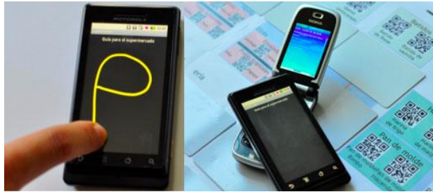
Figure 4 User drawing a “P” (left) on Motorola Milestone, Nokia 6131 NFC to read HF RFID tag for navigation and supermarket mock-up for testing (right)
