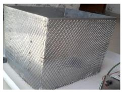
Cooling tower = A air cooled cooling tower is used to cool the hot water. The height of the cooling tower from the base is 65cm. at the top the falls on the smallest plate of the cooling tower and then in form of drops on the medium size plate and finally on the biggest plate. From where it is further carried through pipes to the aluminum box. The cooling tower is made up of galvanizing sheet of thickness 22 gauge.
