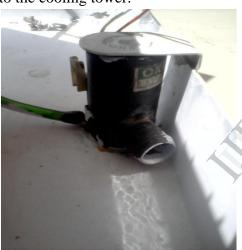
Fan = A 12 volt fan is fitted on the wall of the insulating plate which air inside regulates the aluminium box through holes on the aluminium box.
