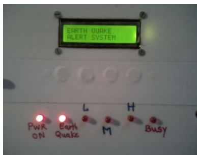
Fig.5 System display indicating earthquake
