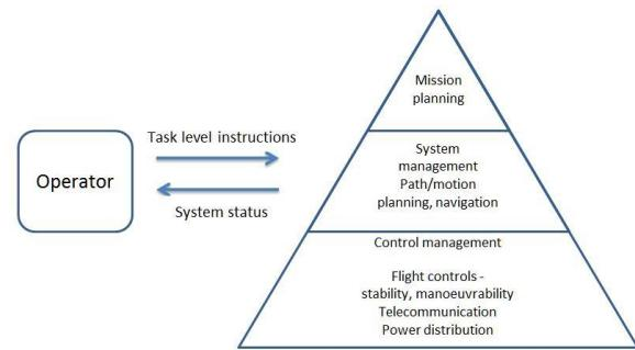
ICAO classifies uncrewed aircraft as either remotely piloted aircraft or fully autonomous. Actual UAVs may offer intermediate degrees of autonomy. E.g., a vehicle that is remotely piloted in most contexts may have an autonomous return-to base operation.
