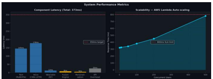
Fig. 5. System Performance — Component Latency and AWS Lambda Scalability
