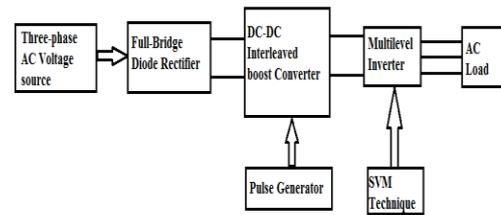
Figure 3. Block diagram of the proposed topology of multilevel inverter
