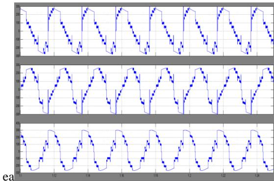
Figure 12. Nine-level output voltage of the proposed model
