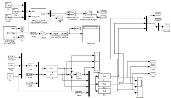
Figure 7. Block diagram of SVM technique employed in the proposed topology
