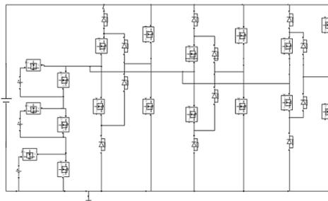
Figure 6. Circuit diagram of MLI used in the proposed model
