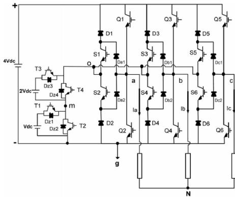
Figure 2. Circuit diagram of the existing multilevel inverter
