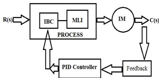
Figure 8. Block diagram of Closed-loop structure
