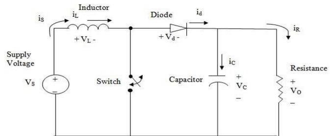
Figure 4. Basic schematic diagram of the Boost converter
