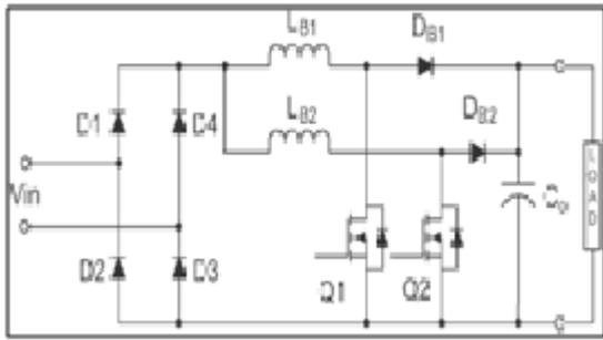
Figure 5. Schematic diagram of the interleaved phase-shift boost converter
