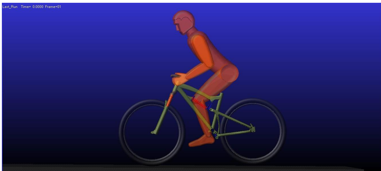
Fig. 6. Position of front and rear spring-damper system in mountain bike.
