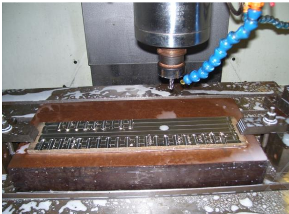
Fig 1: Fixation of AISI 304 stainless steel plate by using clamps in the machining center
