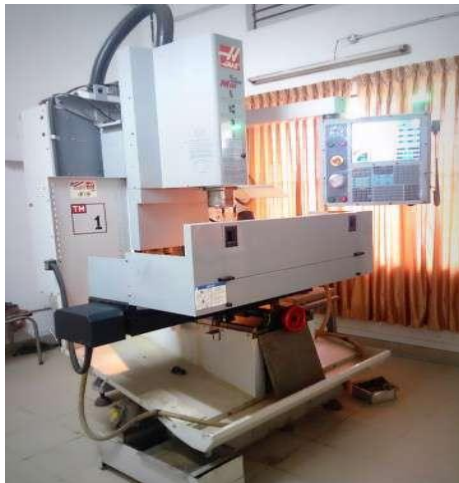
Figure:1 HAAS CNC Vertical Tool Room Mill (TM-1)
