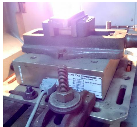
Figure 4: Unitech Milling Tool Dynamometer (UIMD-14)
