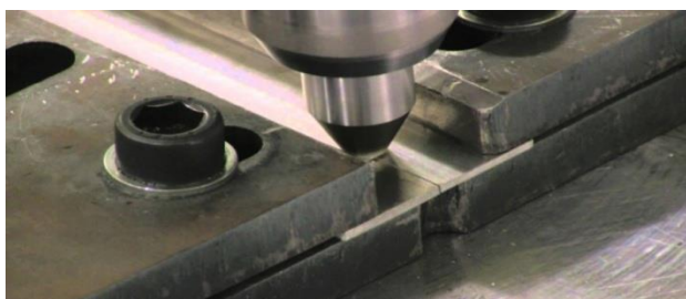
Fig. 3: clamped plates of FSW
