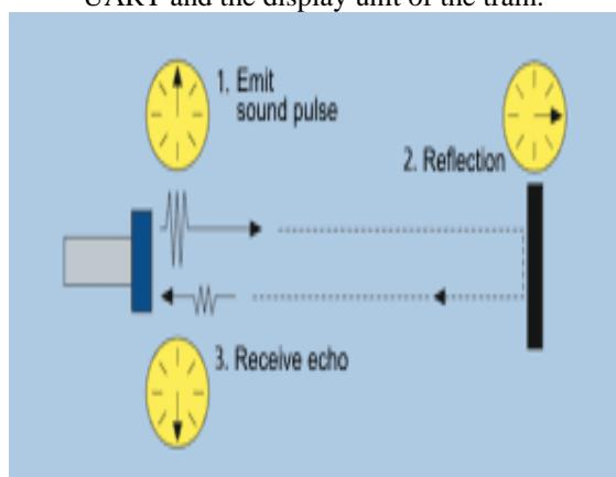
The above diagram shows the working of ultrasonic sensors where the sound pulse is given out by the sensors at a specific frequency and they receive the echo. Thus the distance is calculated by the time elapsed between generated and the received sound wave.
