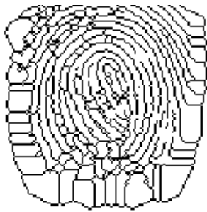
Fig.8. Fingerprint minutiae feature extracted
