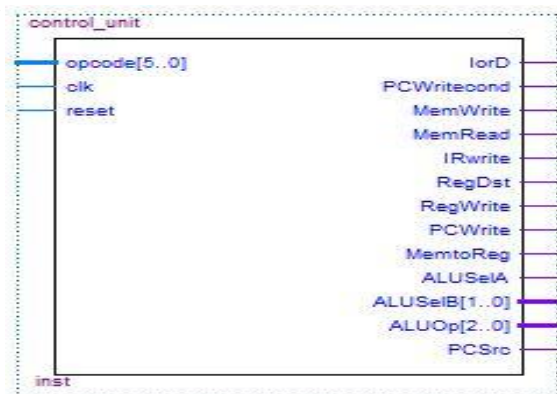
Fig. 7. Block diagram of CONTROL UNIT
