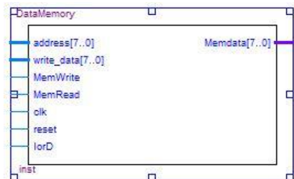
Fig. 8. Block diagram of DATA MEMORY.
