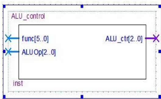
Fig. 9. Block diagram of ALU CONTROLLER
