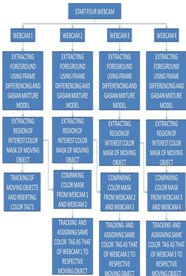
Fig. 5. Flow chart of object detection and tracking using four Webcam
