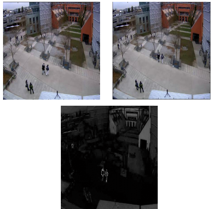
Fig 4.Foreground regions obtained using image difference scheme: (a) the kth frame, (b) the transformed (k -1) th frame, and (c) obtained foreground regions.
