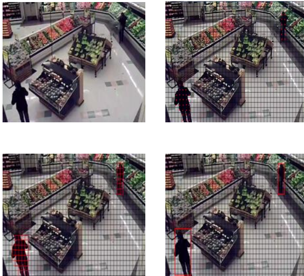
Fig.2 Fruit and vegetable store (a) Original Frame (b) Result of motion detection (c) Result of clustering algorithm (d) Motion area in frame.
