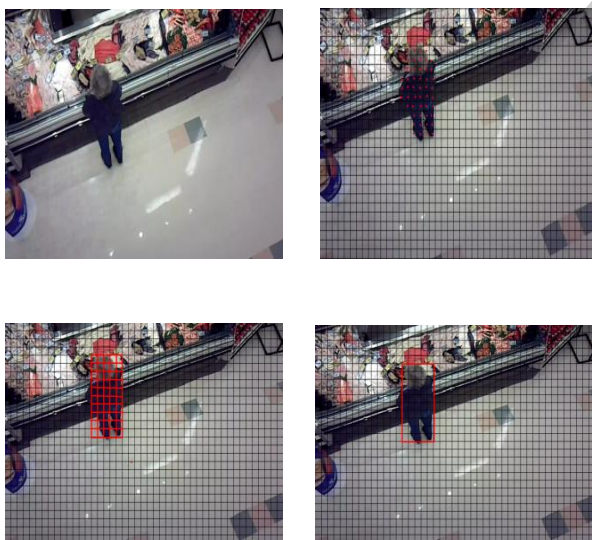
Fig.3 Super store (a) Original Frame (b) Result of motion detection (c) Result of clustering algorithm (d) Motion area in frame.
