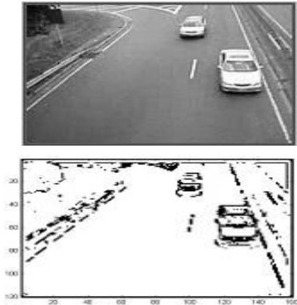
Fig 2: a) gray-scale image b) Thresholded image
