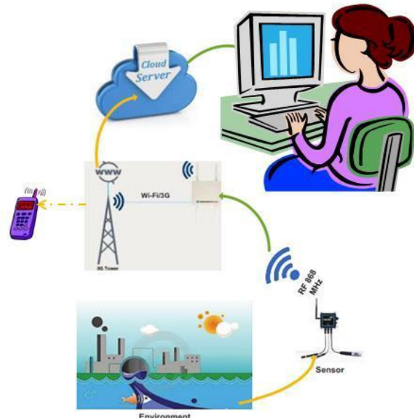
Fig 3.Proposed system for smart water analysis in an IoT Environment
