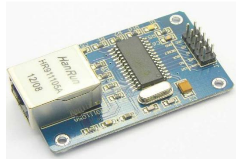
Figure 3. Ethernet Controller ENC28J60
