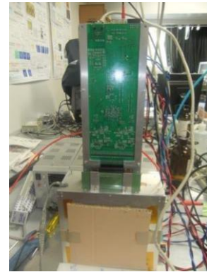
Figure 4 Epithermal Neutron Imaging Camera with GEM at Nagoya University, Japan
