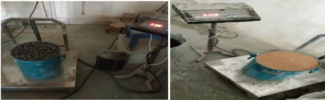
FIGURE 3.40 Bulk and Packing Density of Aggregate
