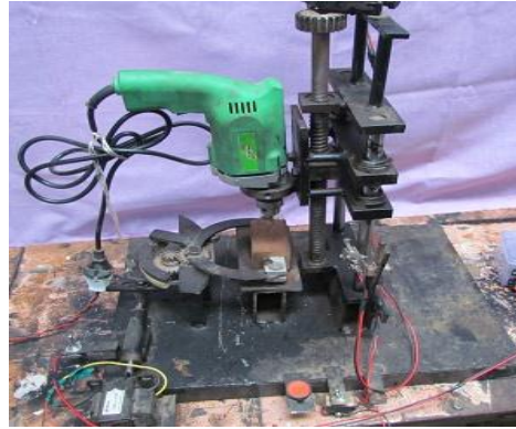
Fig 4 Experimental set up of drilling machine
