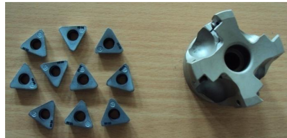
Fig. 2 Cutting inserts and the milling cutter
