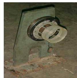
Figure 5 Stress freezing arrangement with fixture and applied load
