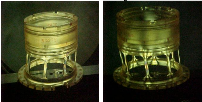
Figure 6 Stress Frozen Model Viewed in a Polariscope The isochromatic fringe pattern for different flex webs is shown in figure 7
