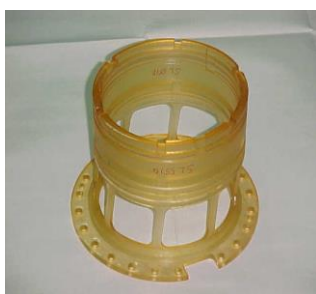
Figure 4 Photo elastic models produced by SLA RP
