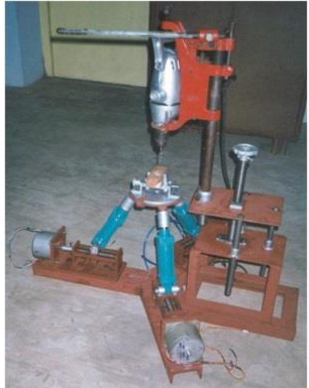
Fig.4 Angular drilling machine with triglide mechanism
