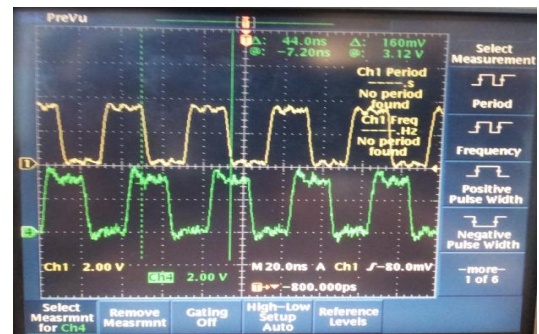
Figure 6 (b) comparison of the waveshapes, yellow waveshape(upper) represent for proposed board and green (lower) for standard board.
