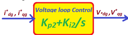
Fig. 6. PI controller tuner for GSC voltage control.
