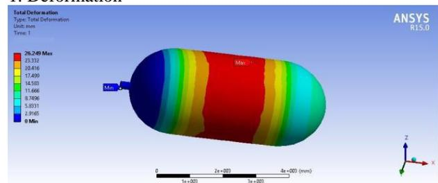
Fig. 11. Static Structural Deformation of Epoxy e-Glass
