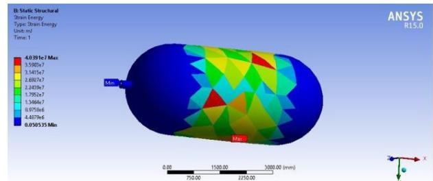
Fig. 10. Static Structural Strain Energy of Epoxy s-Glass
