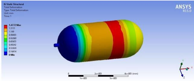
Fig. 5. Static Structural Deformation of Steels515-gr70
