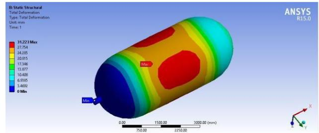
Fig. 8. Static Structural Deformation of Epoxy s-Glass
