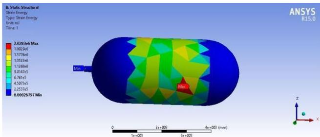
Fig. 7. Static Structural Strain Energy of Steels515-gr70
