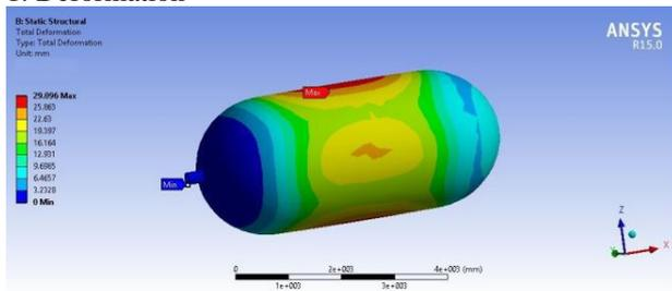
Fig. 14. Static Structural Deformation of Epoxy Carbon
