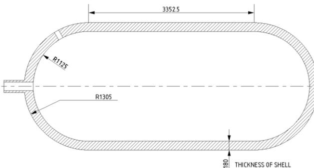
Fig. 1. Line Diagram of the Pressure Vessel
