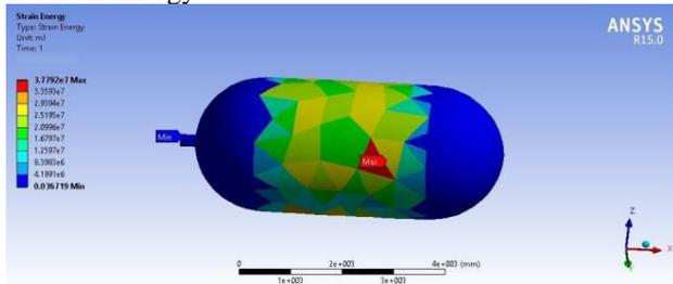
Fig. 13. Static Structural Strain Energy of Epoxy e-Glass
