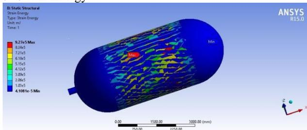
Fig. 19. Static Structural Strain Energy of Steel-s515-gr70 and Epoxy Carbon
