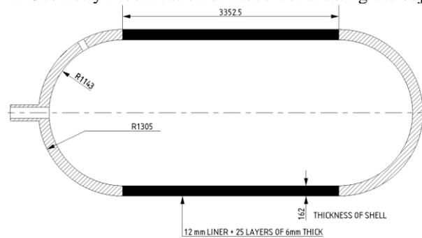
Fig. 17. Line Diagram of the Multi-layered Composite Pressure Vessel
