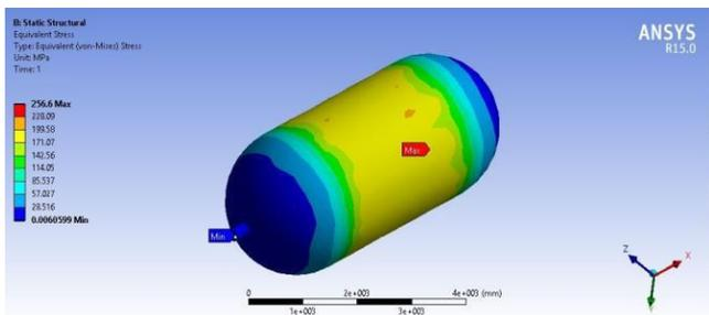
Fig. 6. Static Structural Von-Mises stress of Steels515-gr70
