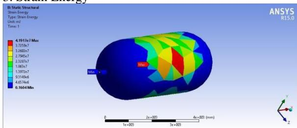
Fig. 16. Static Structural Strain Energy of Epoxy Carbon
