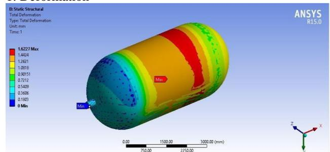
Fig. 17. Static Structural Deformation of Steel-s515-gr70 and Epoxy Carbon
