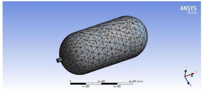
Fig. 3. FE Tetra-Mesh of Pressure Vessel in Ansys Workbench
