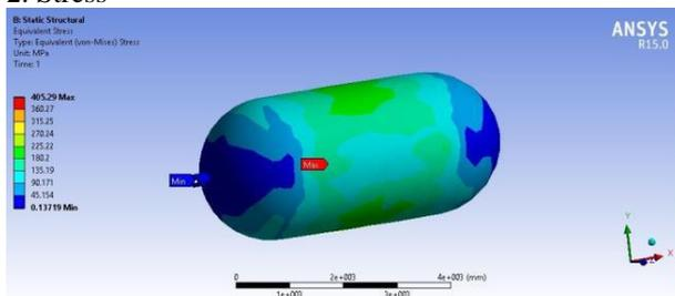
Fig. 15. Static Structural Von-Mises stress of Epoxy Carbon
