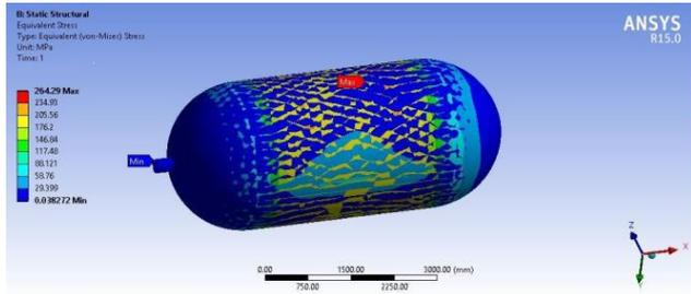
Fig. 18. Static Structural Von-Mises stress of Steel-s515-gr70 and Epoxy Carbon
