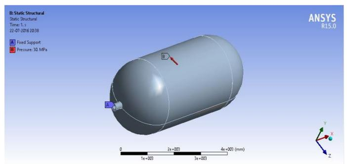
Fig. 4. Boundary Conditions of the Pressure Vessel
