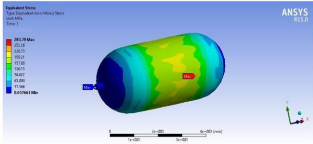
Fig. 12. Static Structural Von-Mises stress of Epoxy e-Glass
