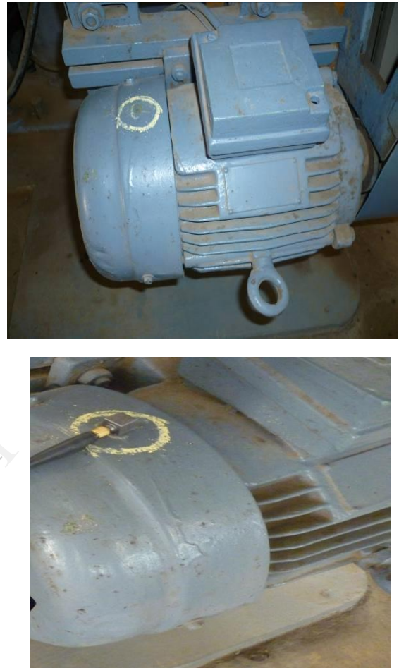
Fig.4 Marking Positions for Accelerometer
