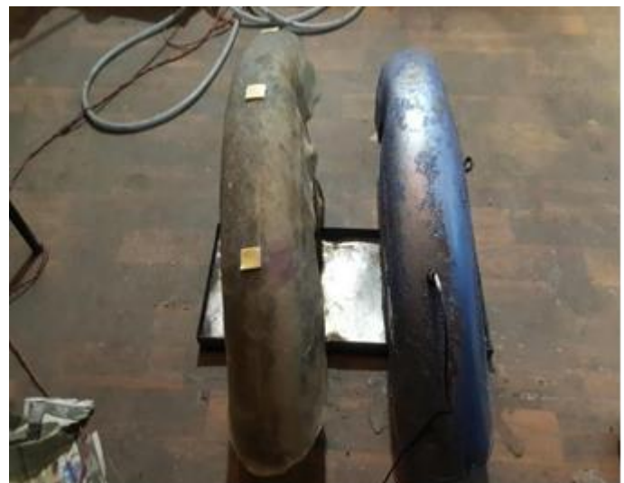
Fig 4 Epoxy resin Glass Fiber and Steel Mudguard
