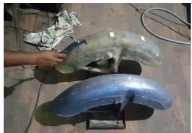
Fig 9 Testing and Validation by Impact Hammer & FFT Analyzer
