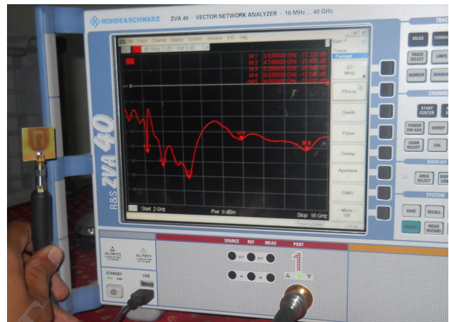
Fig. 14 Set up of antenna measurement using VNA
