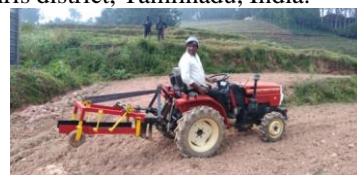
Fig. 7 Potato harvesting machine under field testing at ICAR-CPRS, Ooty
