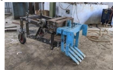
Fig. 1 Vibrating Potato Harvester under fabrication
