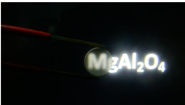
Fig. 6. Photograph of polished \text{MgAl}_2\text{O}_4 pellet placed 2mm above computer screen
