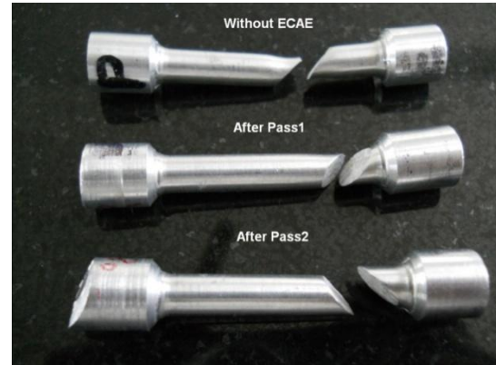
Fig.5 Fractured specimens after tensile test
