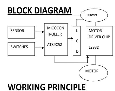
Based on sensor and switch polling method in which observation of changes made over switches done by sensors through messege
