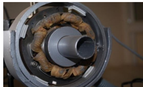
Fig.1. the physical arrangement of Stator & Rotor of AMB.
