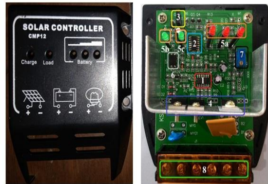
Fig. 3. PWM Solar Charger Controller, 12V-10A
