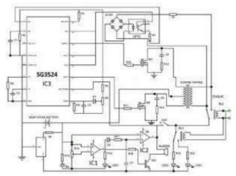
fthe type of load connected. This can be achieved by changing the switching frequency width at the oscillator.
