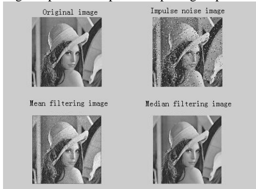
Fig.4. Results with impulse noise , by mean filtering and median filtering
