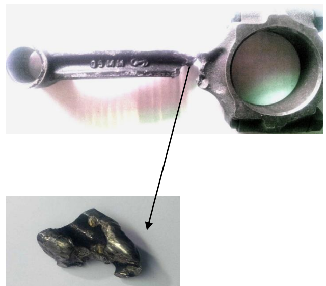
Fig.1 Fractured Connecting Rod and Specimen according to SEM tool Holder
