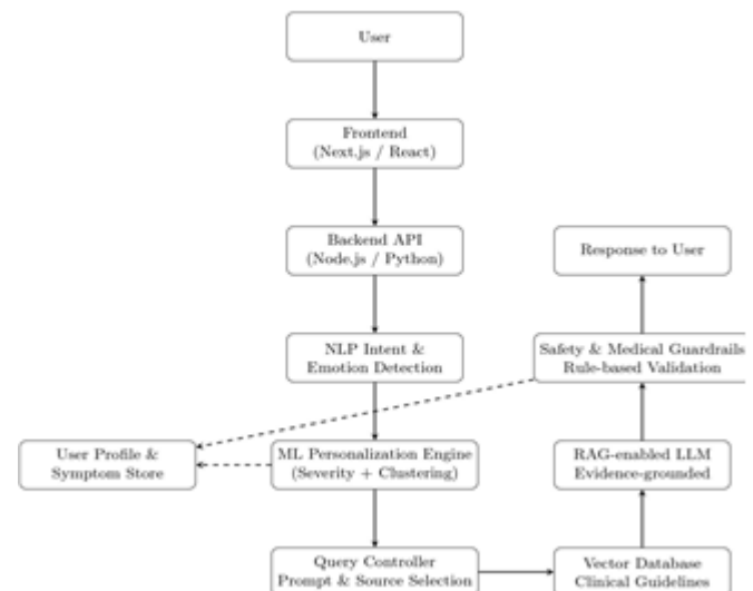
Figure 1: Modular AI system architecture of MenoEaze integrating intent and emotion detection, personalization, and RAG over clinical knowledge sources.
