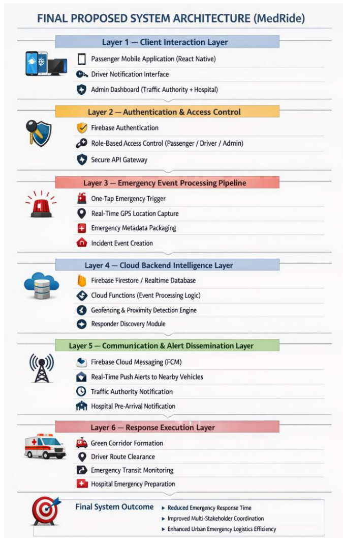
Fig. 1. System Architecture of MedRide for Layered Emergency Response Coordination
