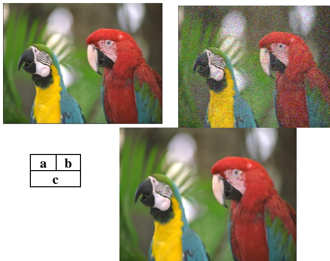
Fig 2: a) Original Image b) Image corrupted by 10% impulse noise c) Restored image using median filter.
