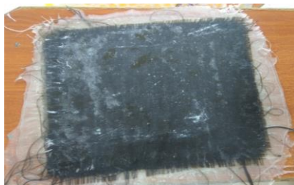
Fig : 5 Applying Epoxy resin of Glass and Basalt fibre
