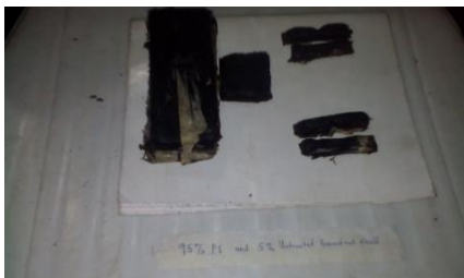
95% POLYETHYLENE & 5% REINFORCEMENT BLENDED
