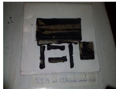
90% POLYETHYLENE & 10% REINFORCEMENT BLENDED
