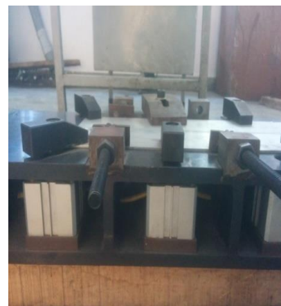
Fig 4: Pneumatic fixture for FSW joint
