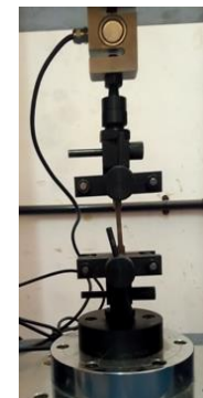
Fig 7: Tension Testing in Universal Testing Machine
