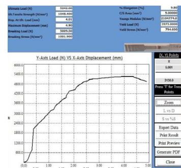
Fig. 8: Tensile test result of Base Metal with specimen
