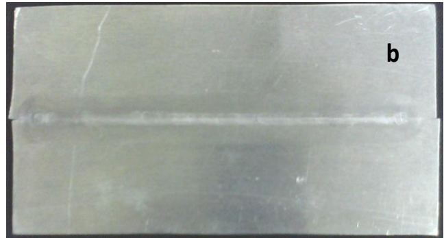
Fig.3 Welded plates by FSW showing (a) top and (b) bottom surface.
