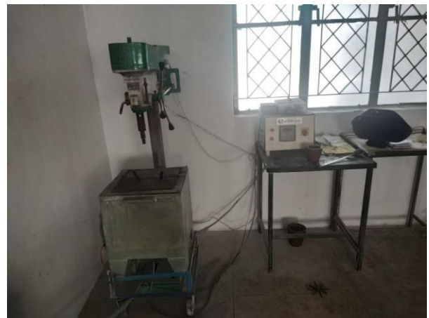
Fig. 2 Schematic of stir casting set-up used for fabrication of Composites
